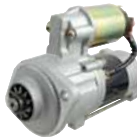
17081N Starter - Mitsubishi OSGR 2.2KW/12 Volts, CW, 11-Tooth Pinion
