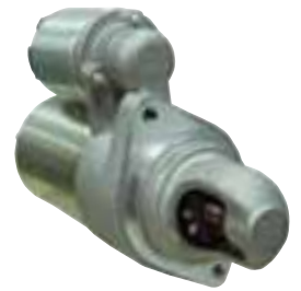
6765N Starter - Delco PMGR 0.8KW/12 Volts, CCW, 10-Tooth Pinion Used on: John Deere Z-Trak model Z830A Pro Kawasaki FX751V 27HP Engines Kawasaki FX850V 31HP Engines Replaces: Delco 8000153; John Deere MIA11257; Kawasaki 21163-7021 Note: Delco PMGR design 6765N can replace Denso DD starter 428000-6610
