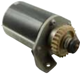
5936N Starter - Briggs & Stratton PMDD 12 Volts, CCW, 24-Tooth Pinion Used on: Briggs & Stratton Intek 5-7hp Horizontal Shaft Engines Replaces: Briggs & Stratton 694504
