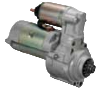
17096N Starter - Mitsubishi OSGR 2.0KW/12 Volts, CW, 13-Tooth Pinion
