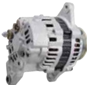
12077N Alternator - Mitsubishi IR/IF 40 Amp/12 Volts, 1-Groove Pulley
