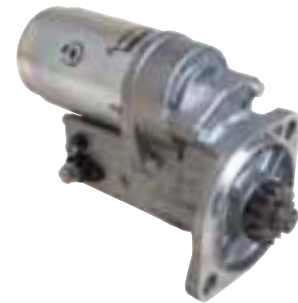
18205N-ND Starter - Denso OSGR Replacement 1.4KW/12 Volts, CW, 15-Tooth Pinion
