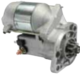
18144N Starter - Denso OSGR 1.4KW/12 Volts, CW, 9-Tooth Pinion
