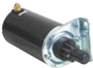
5951N Starter - United Technologies PMDD 12 Volts, CCW, 10-Tooth Pinion Used on: Cub Cadet Mowers w/ 15-23hp Kawasaki Small Engines Kawasaki FH500V, FH531V, FH541V, FH580V, FH601D, FH601V, FH641D, FH641V, FH661V, FH680D, FH680V, FH721D, FH721V, FH770D Small Engines Replaces: Kawasaki 21163-7001, -7010, -7022, -7029
