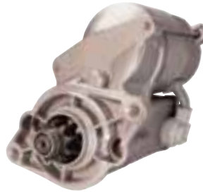
17028N Starter - Denso OSGR 1.0KW/12 Volts, CW, 9-Tooth Pinion
