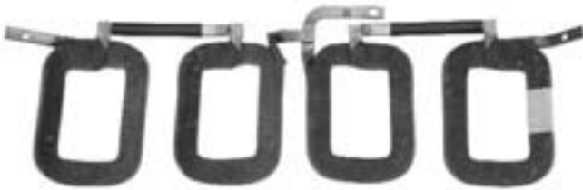
59-304 Field Coil 12 Volt, CW Rotation
