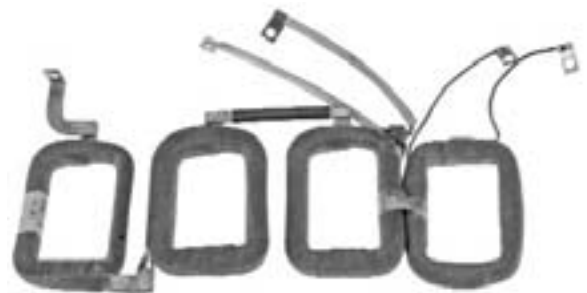
59-160 Field Coil 12 Volt, CW Rotation
