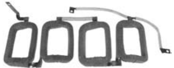
59-153 Field Coil 12 Volt, CCW Rotation
