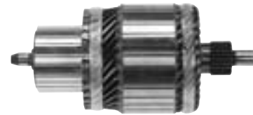
61-137 Armature 12 Volt, CW Rotation
